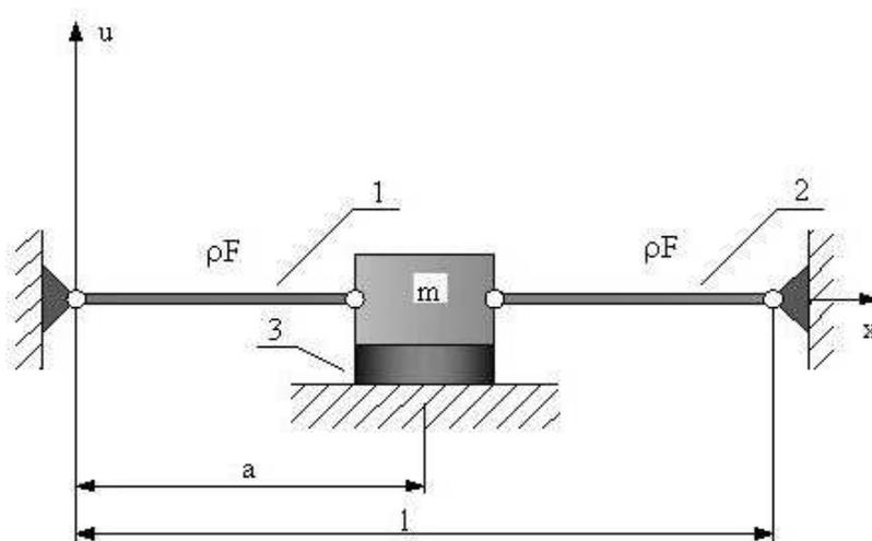
Fig. 9. The model of the vibroinsulation system for the railway crossing
