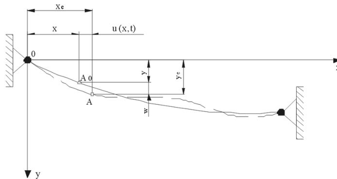
Fig. 10. Displacement of the point on the flexible tension member during the vibration in the plane of hanging
