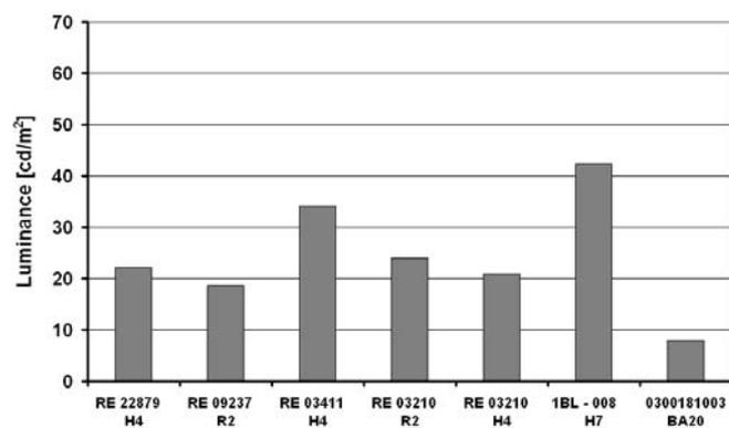
Fig. 29. Luminance values within Area 2 for the examined reflectors and projector
