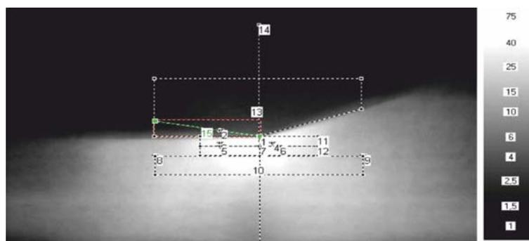
Fig. 4. The view of a light spot of low beam light projector 1BL-008 (H7) together with indicated places of luminance measurement
