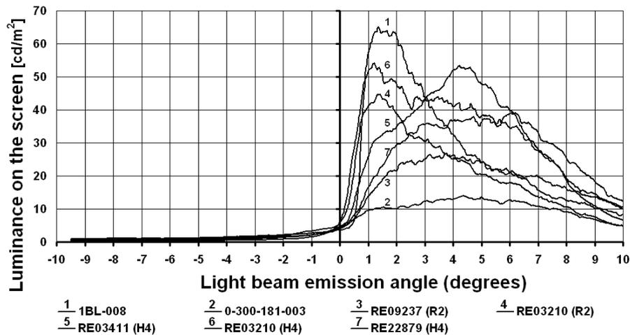
Fig. 32. Section within vertical axis V-V of light beam – borderline of light and shade
