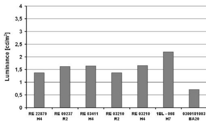
Fig. 30. Luminance values within Area 3 for the examined reflectors and projector
