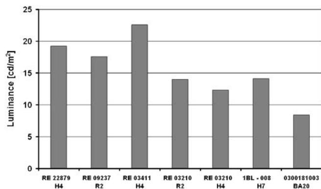
Fig. 20. Luminance values at the point 25R for the examined reflectors and projector
