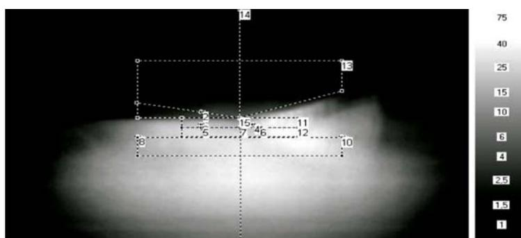
Fig. 12. The view of a light spot of low beam light reflector RE22879 (H4) together with indicated places of luminance measurement
