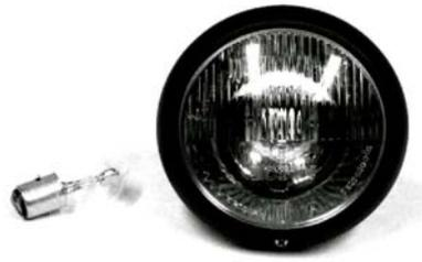
Fig. 5. Main light and low beam light reflector of 0-300-181-003 type with BA20D light bulb
