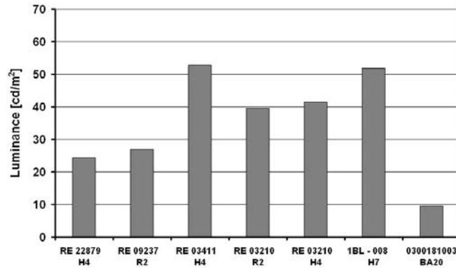
Fig. 22. Luminance values at the point 50R for the examined reflectors and projector
