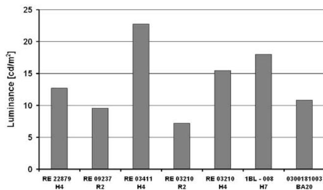
Fig. 19. Luminance values at the point 25L for the examined reflectors and projector
