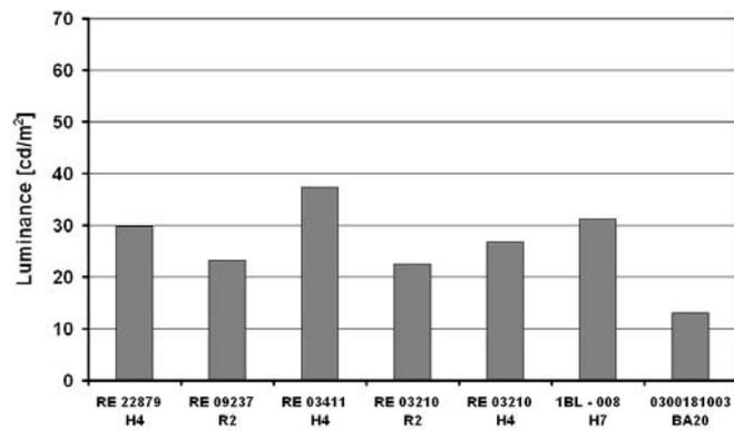
Fig. 28. Luminance values within Area 1 for the examined reflectors and projector
