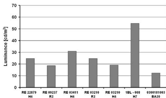
Fig. 21. Luminance values at the point 50L for the examined reflectors and projector
