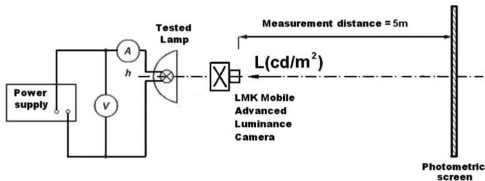
Fig. 2. Measurement station diagram
