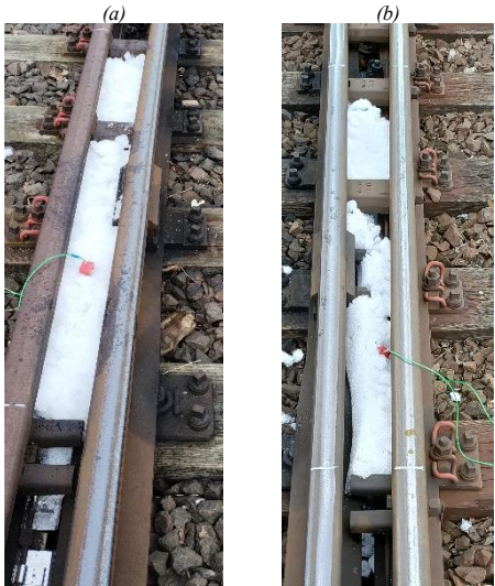
Fig. 4. View of the location of thermoelectric sensors installed on the studied switches No. 38 (a) and reference switch No. 39 (b) in the area covered with snow
