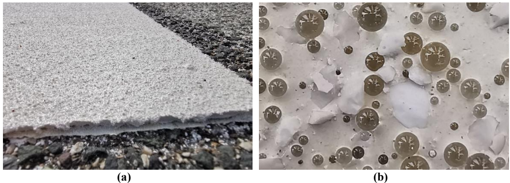
Fig. 1. External appearance of flat line road markings: (a) Side view of flat line circa 3 mm thick; (b) Top close-up view with visible GB and ASP. Source: Author
