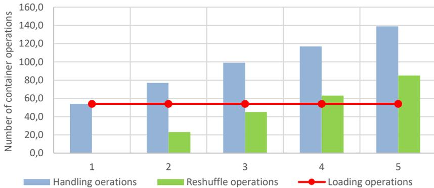
Fig. 6. Number and types of operations performed by the crane during train loading
