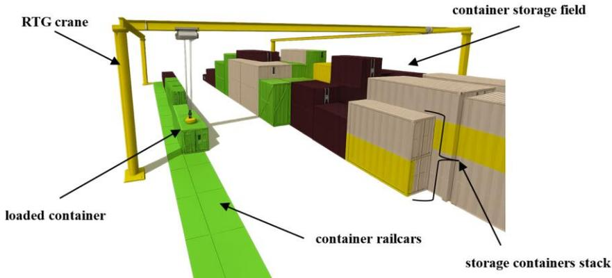
Fig. 3. Container loading front in FlexSim simulation model
