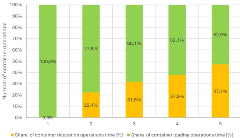
Fig. 8. Share of time spent on loading and reshuffling operations
