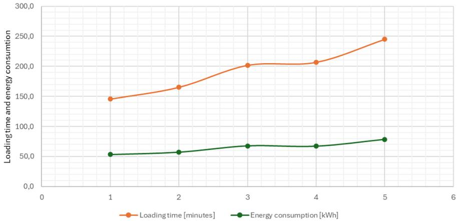
Fig. 5. Results of loading time and Energy consumption by RTG crane
