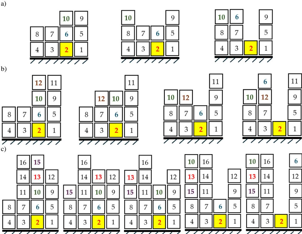
Fig. 2. Containers reshuffling depending on the number of stacking layers a) 3 layers, b) 4 layers, c) 5 layers
