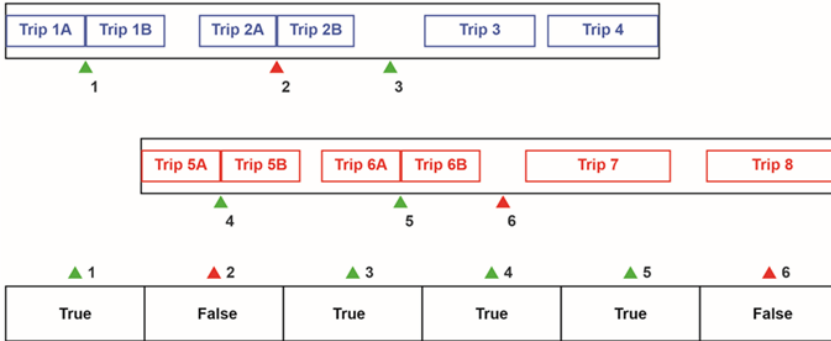
Fig. 1. Vehicle blocks divided into pieces of work (up) based on relief-points defined in the chromosome with six genes (down)
