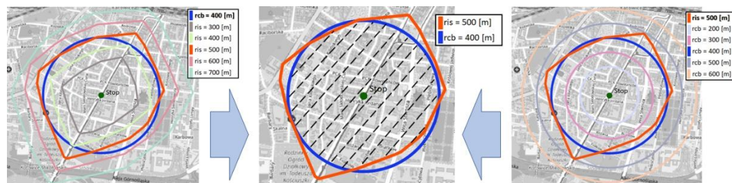
Fig. 5. Visualization of the results of the analysis for the public transport stop pts = 5 , the circular buffer with the radius of rcb = 400 m and the isodistance with the value of ris = 500 m
