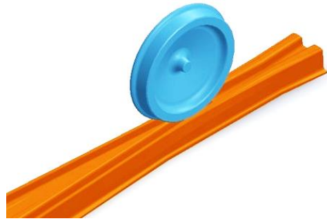
Fig. 2 . Movement of the wheel along the frog of the railroad switch
