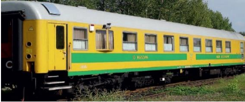
Fig. 5. Ultrasound railroad testing car (Ciszewski, 2007)
