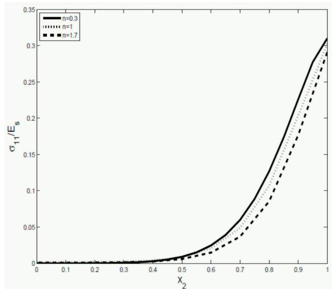
Fig. 6. Through – thickness stress  $\sigma_{11}$  at  $x_1=0$
