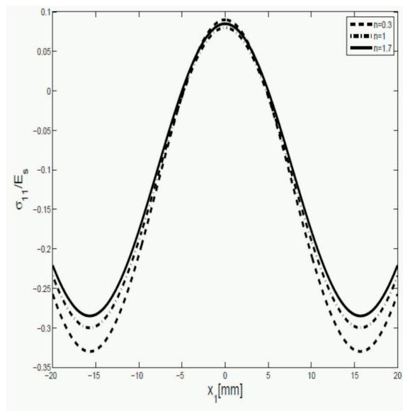
Fig. 9. Longitudinal stress  $\sigma_{11}$  on  $x_2=1$
