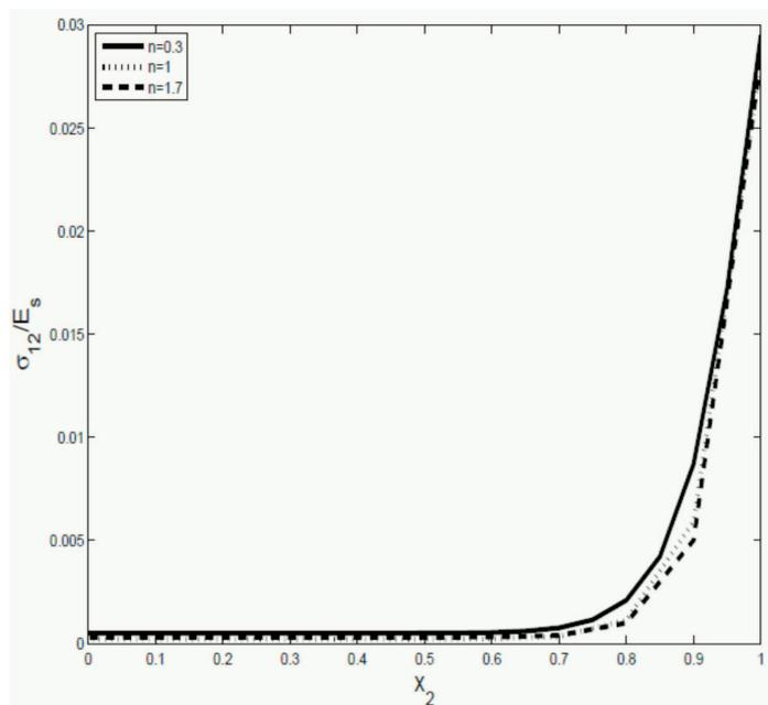
Fig. 7. Through – thickness stress  $\sigma_{12}$  at  $x_1=0$
