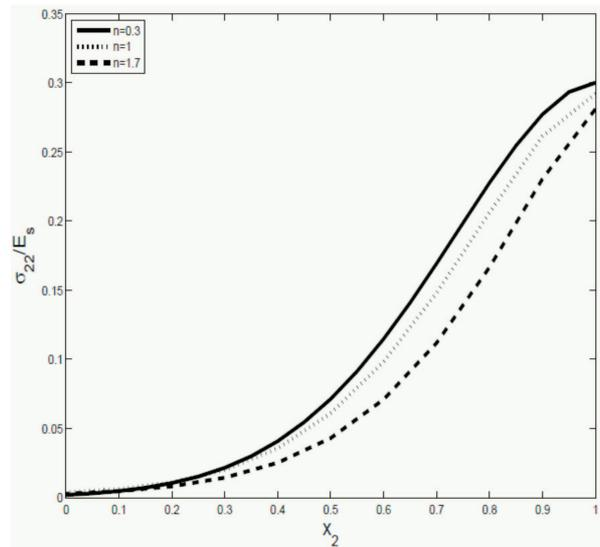
Fig. 5. Through – thickness stress  $\sigma_{22}$  at  $x_1 = 0$
