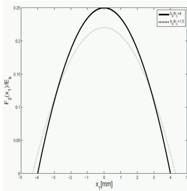
Fig. 4. The dependance of normal contact pressure on thickness ratio  $h_s/h_c$
