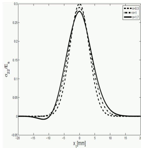
Fig. 8. Longitudinal stress  $\sigma_{22}$  on  $x_2=1$
