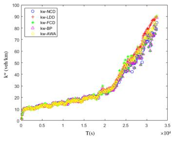
Fig. 4. Comparison of the road network weighted traffic densities obtained by various estimation methods
