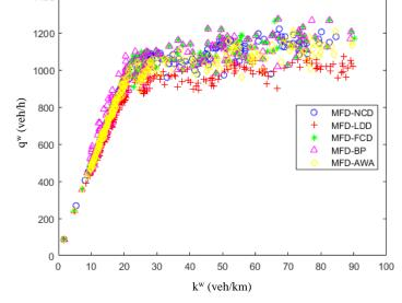
Fig. 6. The two dimensional MFD of road network obtained by various estimation methods
