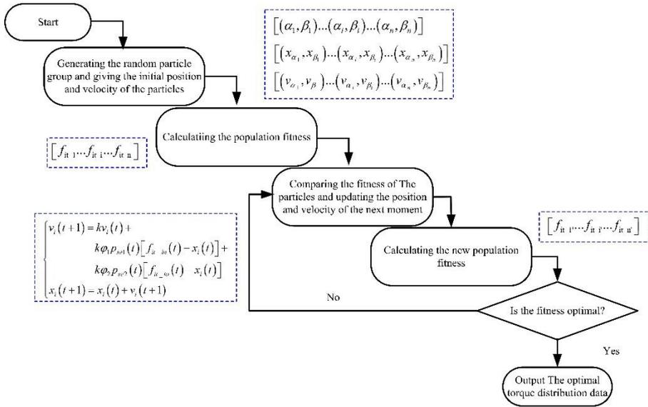
Fig. 6. Off-line optimization program for brake force distribution based on PSO
