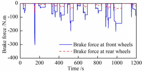
(a) Brake torque distribution ( $\lambda$ ) between front and rear shafts
