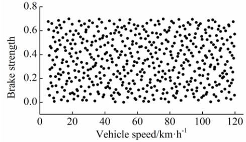
Fig. 5. Two-factor database of brake operation based on HALTON sequence method
