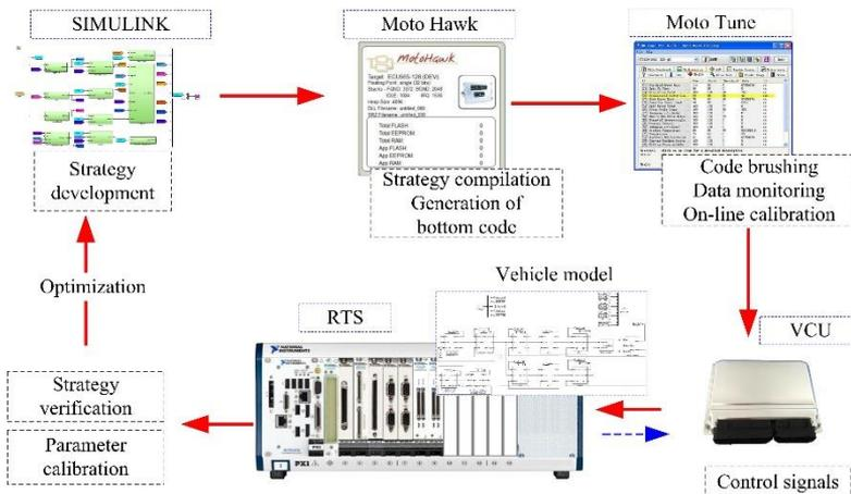
Fig.11. Validation process of the control strategy
