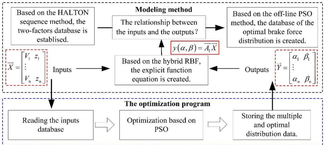
Fig. 3. Multi-objective optimal brake force distribution strategy
