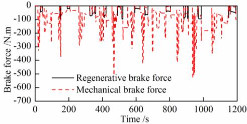
(b) Regenerative and mechanical brake torque distribution ( $\alpha$ )
