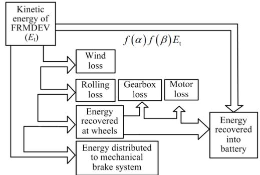
Fig. 1. Characteristic of energy flow during the brake process of FRMDEV
