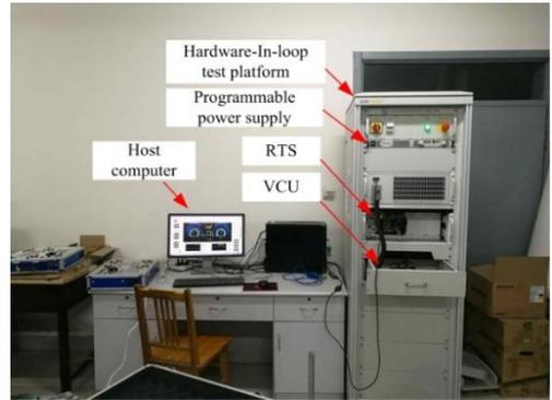
Fig.10. Hardware-in-loop test platform
