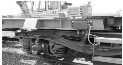
Figure 7. Diagnosis Module Cargo CBM with axle generator and telematic box [5]
