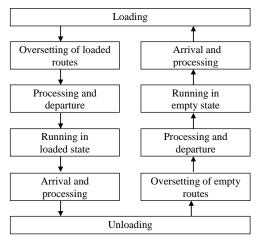
Fig. 3. Schematic diagram of the simulation model of car traffic with grain
