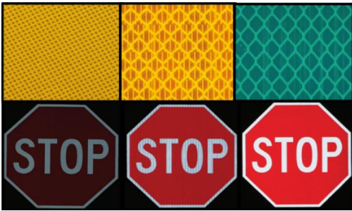
a- Class RA1 b- Class RA2 c- Class RA3 Fig. 3. EN 12899-1:2007 standard traffic sign sheet classes, adapted from (3M Safety Transportation, 2023)
