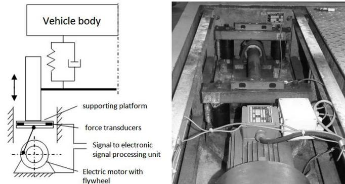
Fig. 3. Test bench working with EUSAMA principle: a) diagram, b) photography of partially disassembled test bench – from the bottom – view of electric motor, flywheel and shaft with a support bearing and with force transducers
