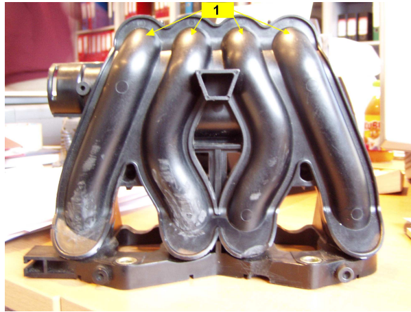
Fig. 3. Factory suction manifold of Fiat 1100 MPI engine: 1 – location of additional injectors were assembled
