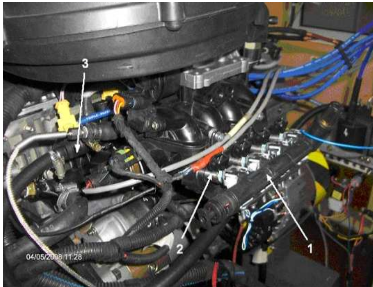
Fig. 4. View of the test bed: 1 – prototype fuel rail, 2 – additional injector, 3 – assembled original, factory fuel rail
