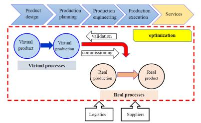
Fig. 1. Twin processes in the Industry 4.0 concept (own study based on Siemens materials)
