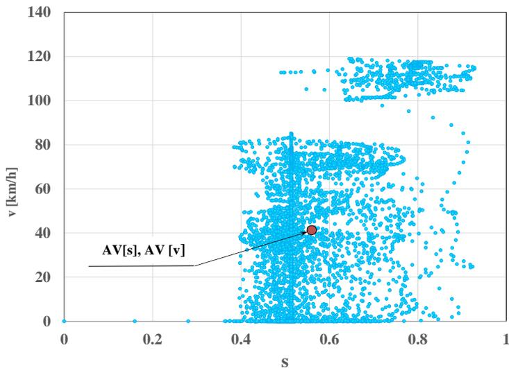
Fig. 12. The relationship between the vehicle speed and the engine control in the RDE test
