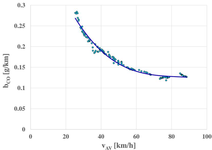
Fig. 16. Carbon monoxide exhaust emission characteristic from the engine of a vehicle in the RDE test
