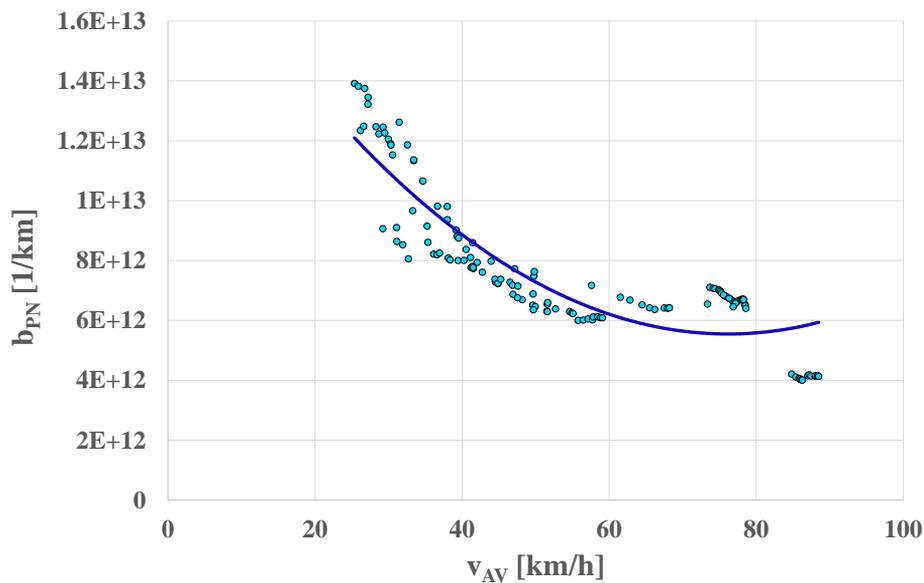
Fig. 20. Particle number exhaust emission characteristic from the engine of a vehicle in the RDE test
