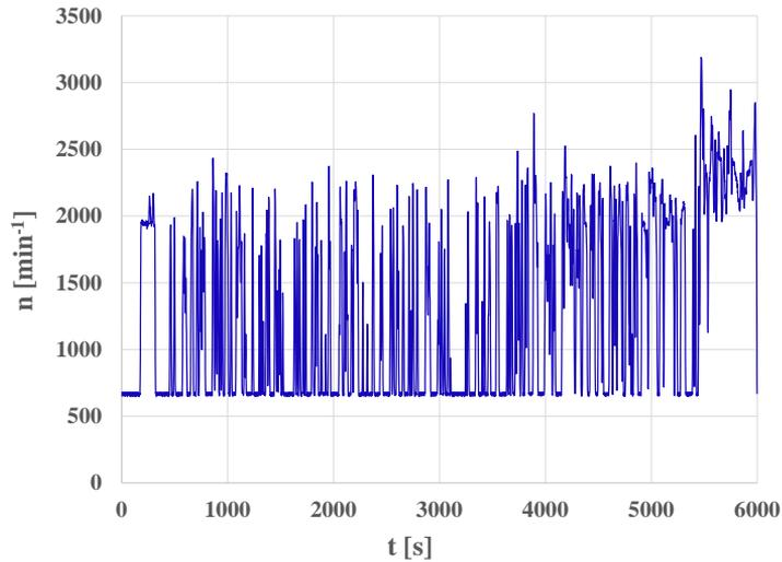
Fig. 3. Engine rotational speed throughout the RDE test
