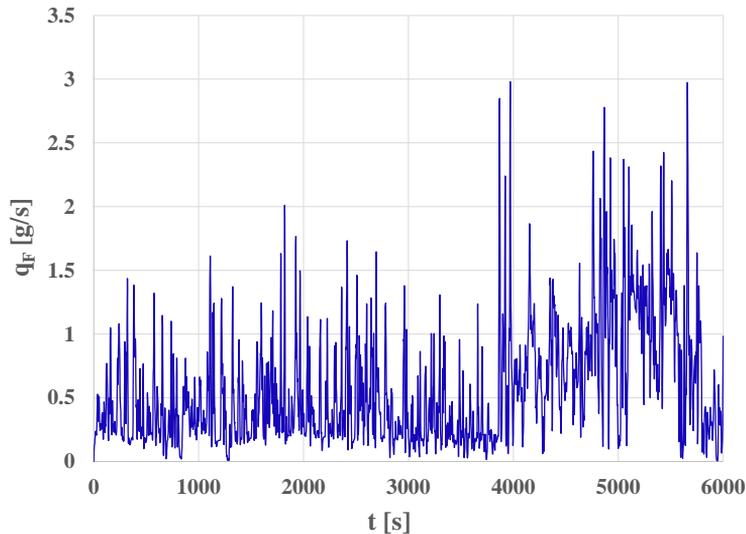
Fig. 11. Fuel mass consumption intensity measured in the RDE test
