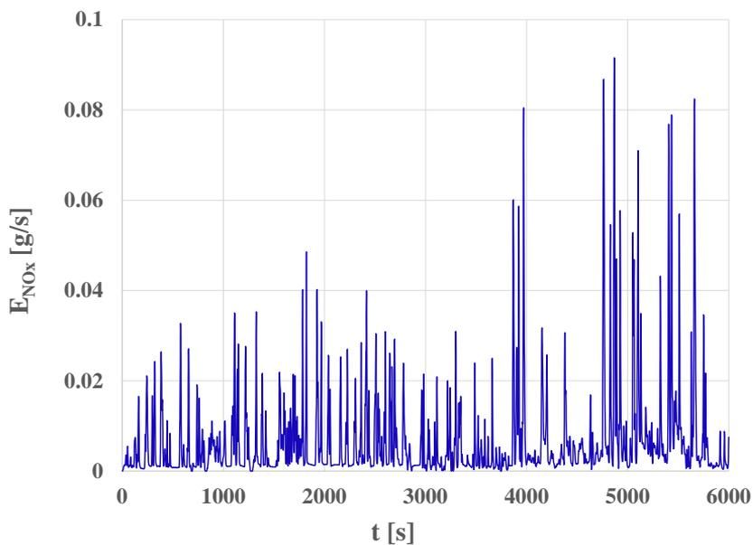
Fig. 8. Nitrogen oxides exhaust emission intensity measured in the RDE test
