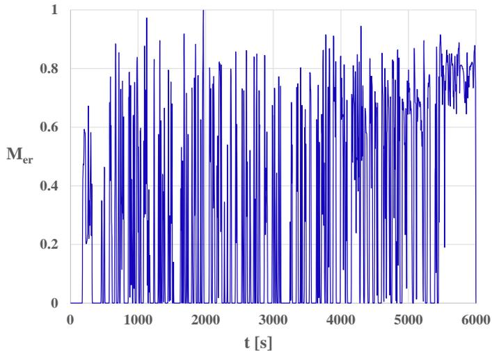
Fig. 4. Relative engine torque during the RDE test
