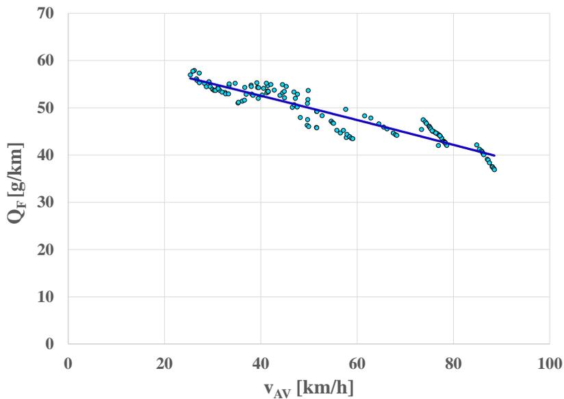
Fig. 21. Fuel mass consumption characteristic from the engine of a vehicle in the RDE test
