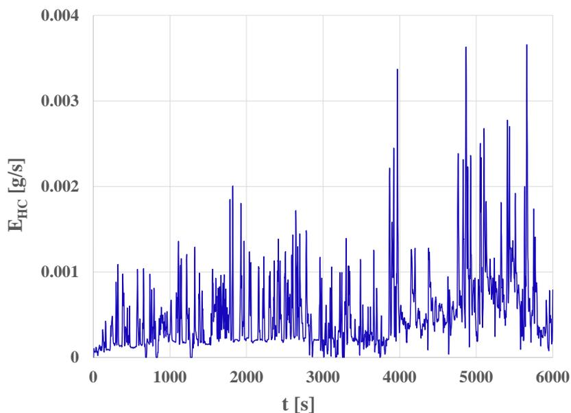
Fig. 7. Hydrocarbons exhaust emission intensity measured in the RDE test
