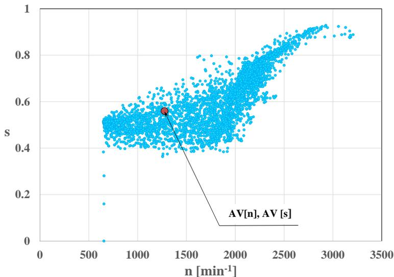
Fig. 13. The relationship between the engine control and the engine rotational speed in the RDE test
