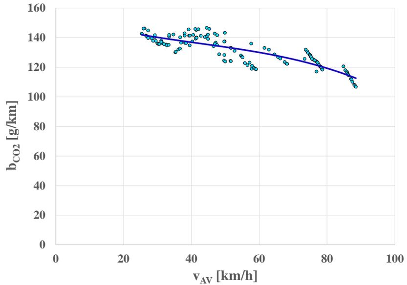
Fig. 19. Carbon dioxide exhaust emission characteristic from the engine of a vehicle in the RDE test
