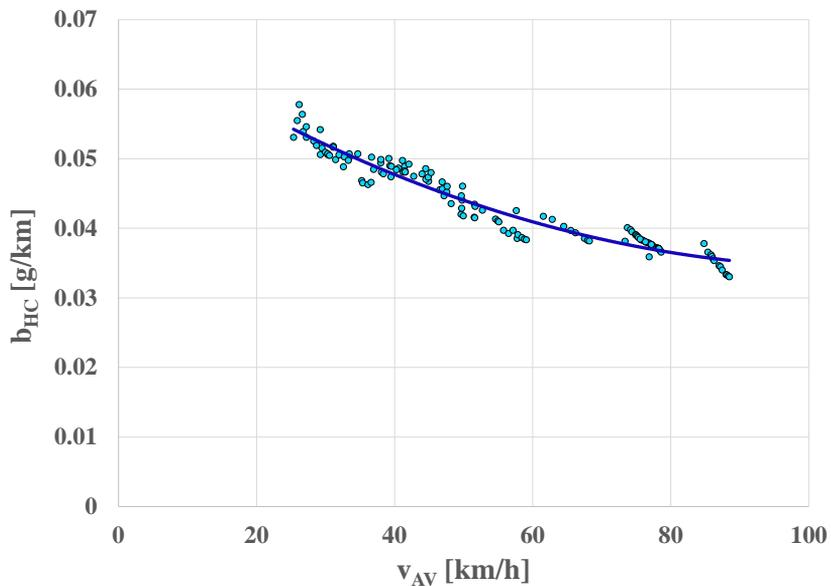
Fig. 17. Hydrocarbons exhaust emission characteristic from the engine of a vehicle in the RDE test
