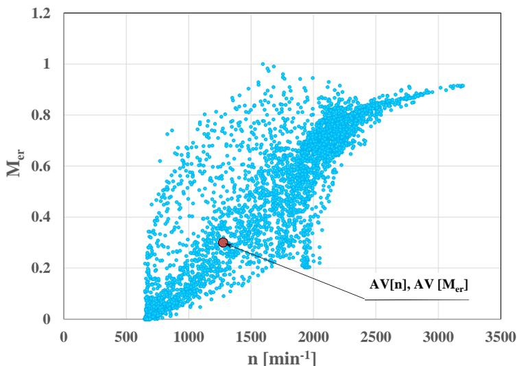
Fig. 14. The relationship between the relative engine torque and the engine rotational speed in the RDE test
