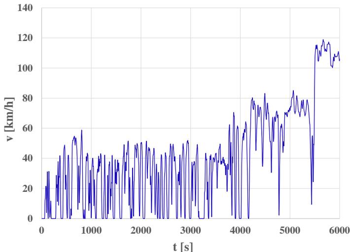
Fig. 1. Vehicle speed profile obtained in the RDE test
