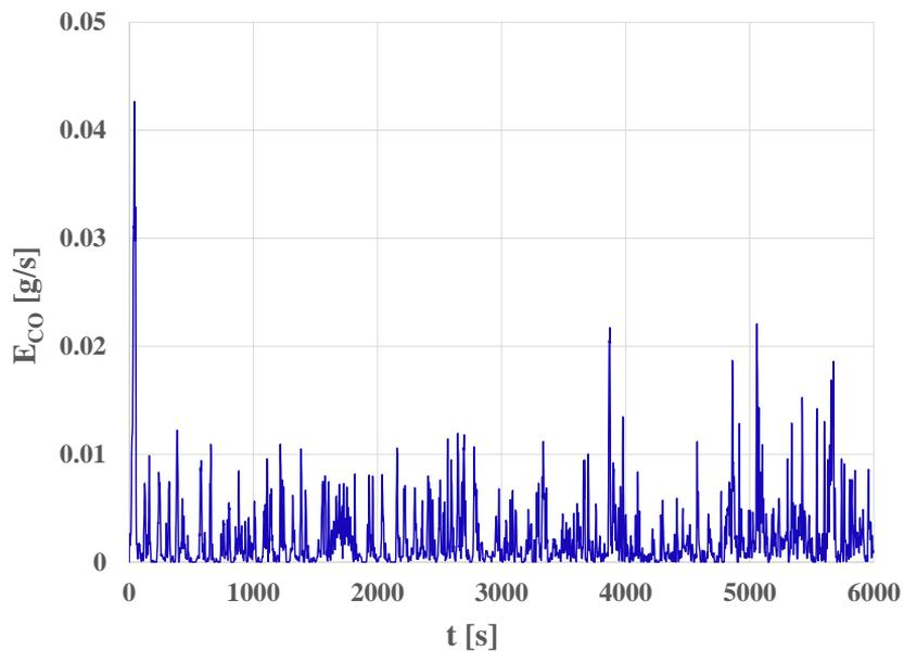
Fig. 6. Carbon monoxide exhaust emission intensity measured in the RDE test
