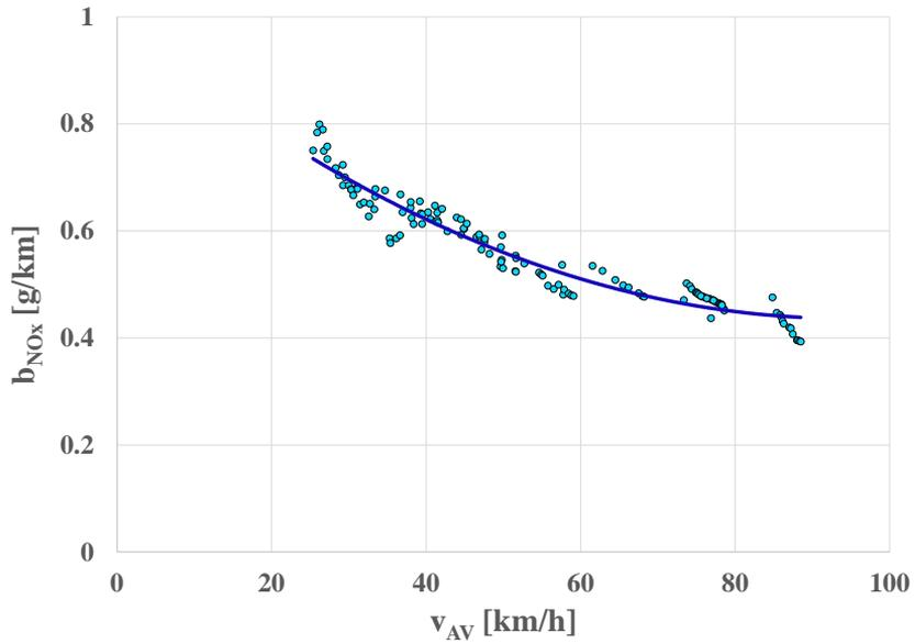
Fig. 18. Nitrogen oxides exhaust emission characteristic from the engine of a vehicle in the RDE test
