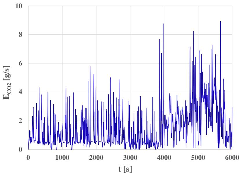
Fig. 9. Carbon dioxide exhaust emission intensity measured in the RDE test
