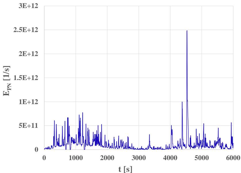
Fig. 10. Particle number exhaust emission intensity measured in the RDE test
