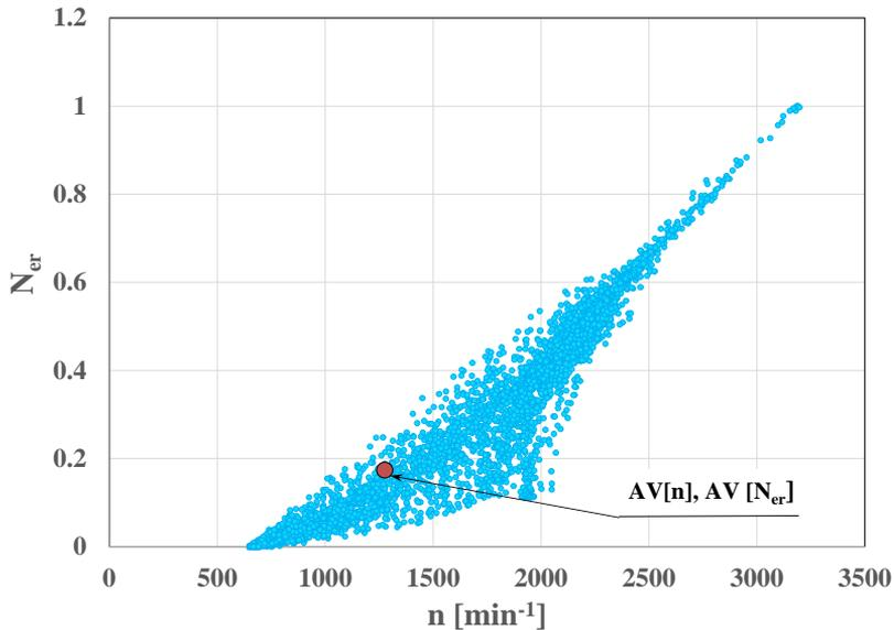
Fig. 15. The relationship between the engine relative net power and the engine rotational speed in the RDE test
