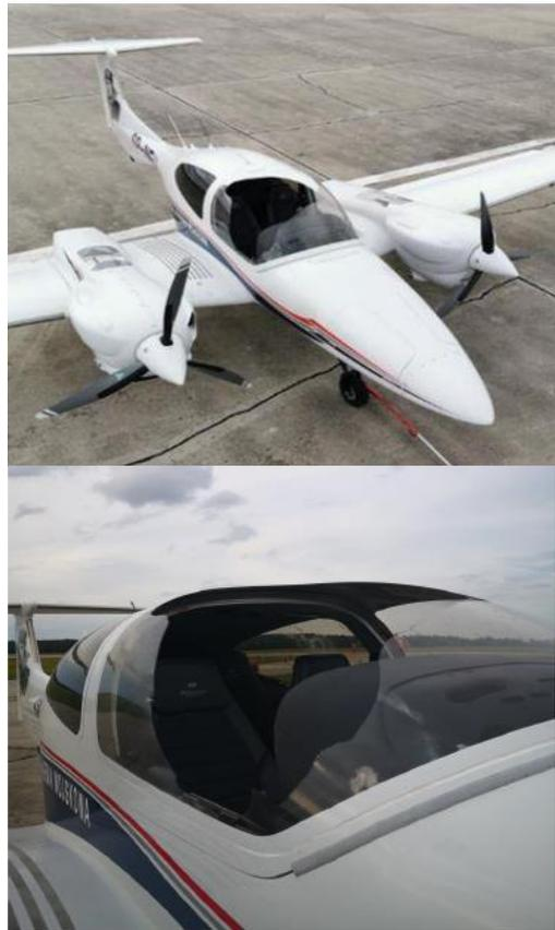
Fig. 1. Damaged windshield of DA-42 after bird strike (courtesy of Marta Kuzyka)
