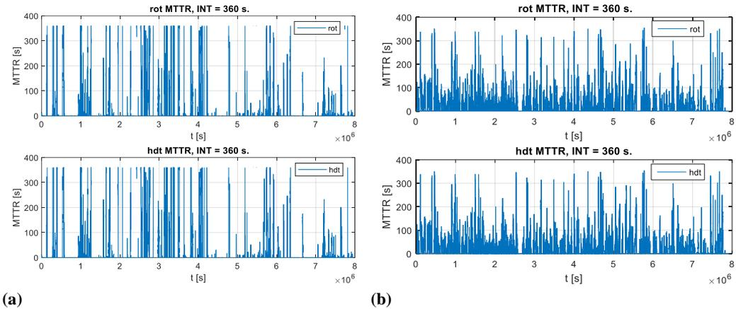
Fig. 8. Mean time to repair based on the age of dynamic data at 360 s intervals for the parameters HDT and ROT, based on the dynamic data recorded by the station (a) PLKOL, (b) PLSWI
