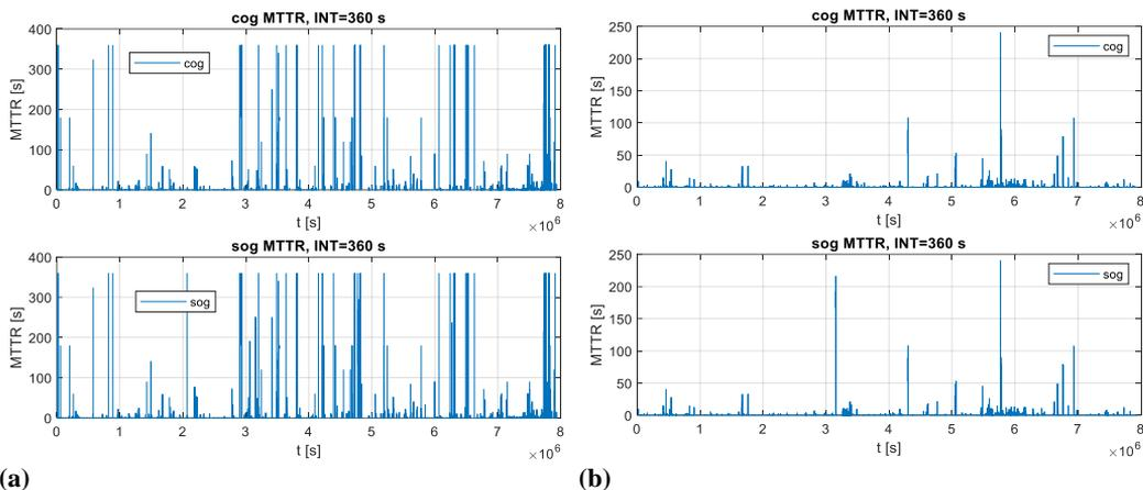
Fig. 6. Mean time to repair based on the age of dynamic data at 360 s intervals for the parameters COG and SOG, based on the dynamic data recorded by the station (a) PLKOL, (b) PLSWI
