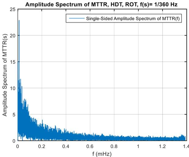
Fig. 17. Single-Sided amplitude spectrum of the mean time to repair for the parameters ROT and HDT, based on the dynamic data recorded by the station PLSZZ
