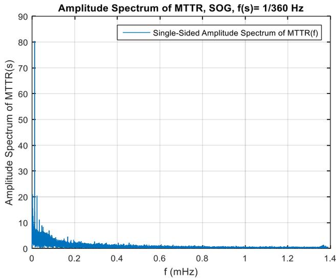
Fig. 15. Single-Sided amplitude spectrum of the mean time to repair for the parameter COG, based on the dynamic data recorded by the station PLSZZ
