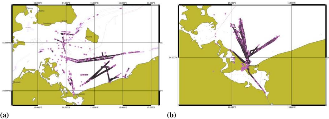
Fig. 2. Geographical positions of the AIS position messages received by the station (a) PLKOL (b) PLSWI
