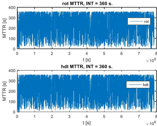
Fig. 9. Mean time to repair based on the age of dynamic data at 360 s intervals for the parameters HDT and ROT, based on the dynamic data recorded by the station PLSZZ
