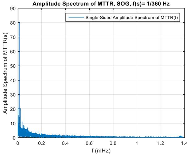
Fig. 13. Single-Sided amplitude spectrum of the mean time to repair for the parameter SOG, based on the dynamic data recorded by the station PLSZZ
