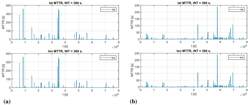
Fig. 4. Mean time to repair based on the age of dynamic data at 360 s intervals for the parameters LAT and LON, based on the dynamic data recorded by the station (a) PLKOL, (b) PLSWI
