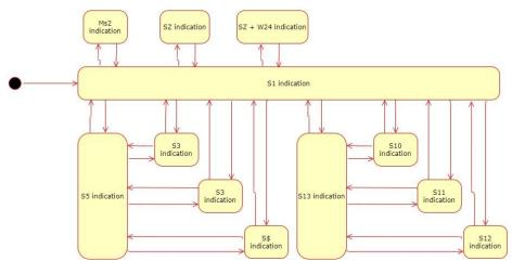
Fig. 3. Example graph representing possible state changes of signals read through LEU encoder. Source: own study
