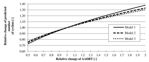
Fig. 2. Relative change of predicted number of crashes with cyclists due to relative change of AADBT
