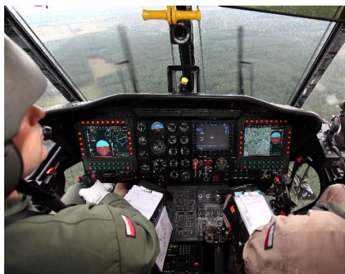
Fig. 2. View of an W3PL cabin with installed MW1 multi-functional screens (Pazur et al., 2019)
