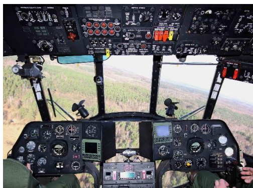
Fig. 1. View of an Mi17 cabin with installed communications control panels PSL1 (Pazur et al., 2019)
