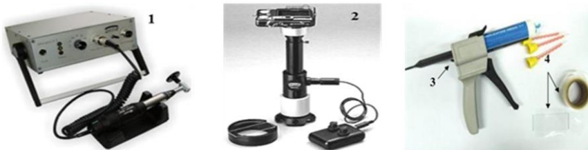
Fig. 7. Equipment for non-destructive metallography: 1 – grinding-and-polishing machine Akkupol; 2 – portable light field microscope TCM; 3 – press for «liquid» replicas; 4 – replicas
