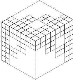
Fig. 3. Fractal particle crushing model
