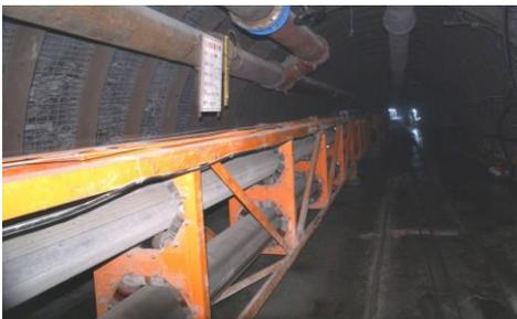
Fig. 1. Chinese first coal mine underground pipe belt conveyor
