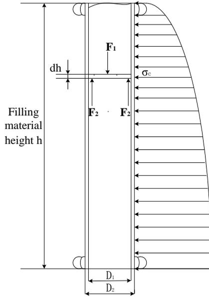
Fig. 2. Pipe belt conveyor lateral stress distribution model
