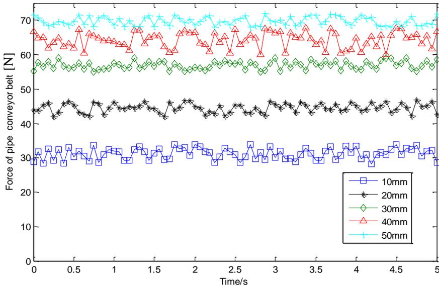
Fig. 5. Simulation graph of the pipe conveyor belt force under different particle sizes
