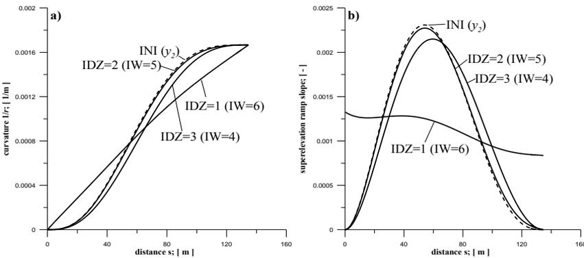
Fig. 7: Route 4 - features of TCs: a) curvatures of the initial and optimised TCs, b) superelevation ramps' slopes
