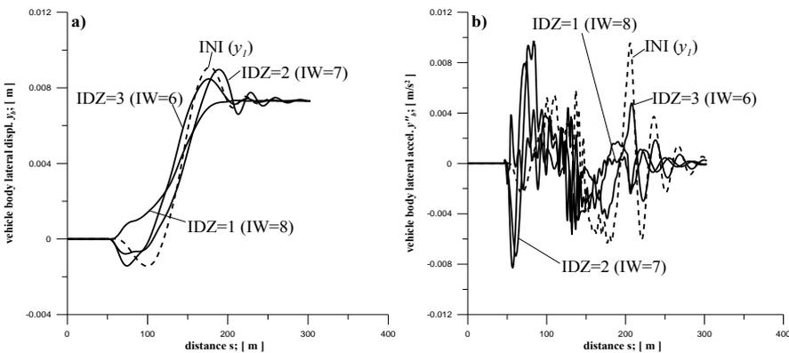
Fig. 10: Route 5 - results of simulation for vehicle body for the initial and optimised TCs: a) lateral displacement, b) lateral acceleration
