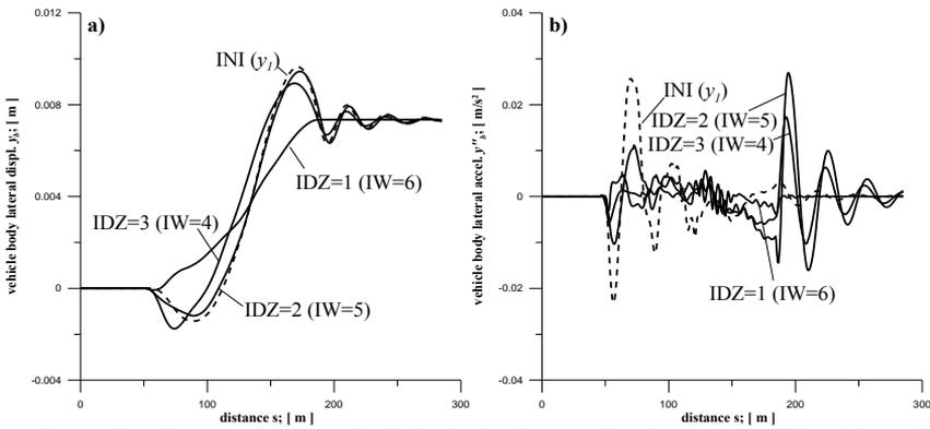
Fig. 6: Route 3 - results of simulation for vehicle body for the initial and optimised TCs: a) lateral displacement, b) lateral acceleration
