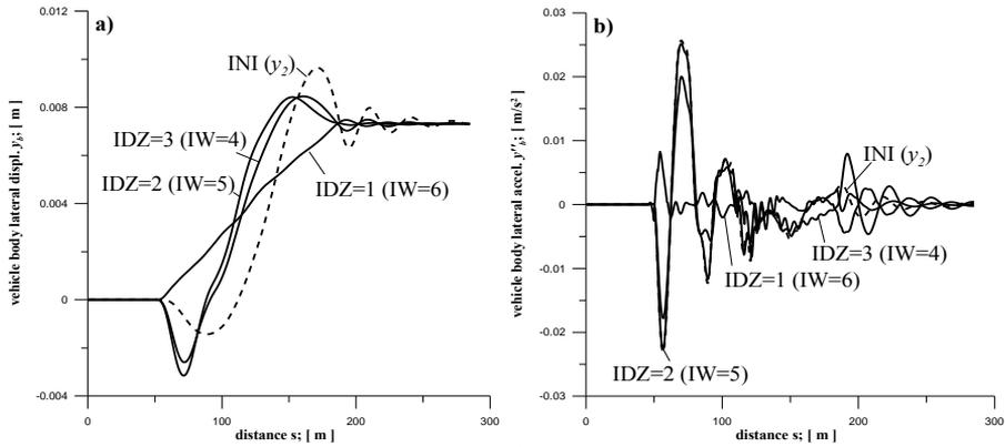
Fig. 8: Route 4 - results of simulation for vehicle body for the initial and optimised TCs: a) lateral displacement, b) lateral acceleration
