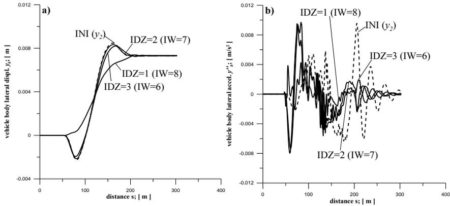
Fig. 12: Route 6 - results of simulation for vehicle body for the initial and optimised TCs: a) lateral displacement, b) lateral acceleration
