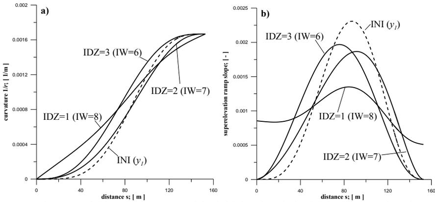
Fig. 9: Route 5 - features of TCs: a) curvatures of the initial and optimised TCs, b) superelevation ramps' slopes
