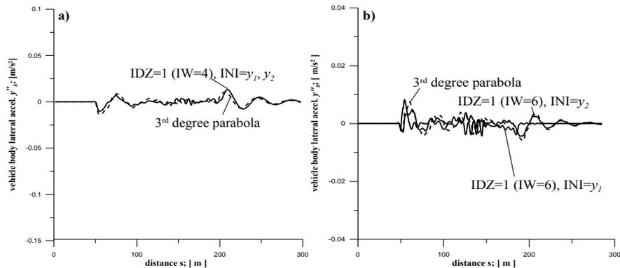
Fig. 13: Results of simulation for vehicle body (lateral acceleration) for the optimised TCs and 3<sup>rd</sup> degree parabola: a) 6<sup>th</sup> (Routes 1 and 2), b) 8<sup>th</sup> (Routes 3 and 4)
