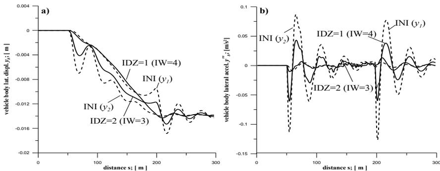
Fig. 4: Route 1, 2 - results of simulation for vehicle body for the initial and optimised TCs: a) lateral displacement, b) lateral acceleration
