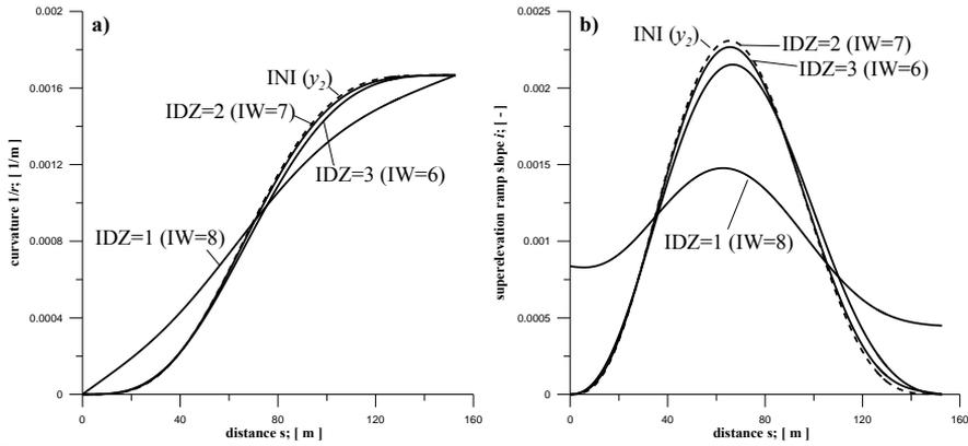
Fig. 11: Route 6 - features of TCs: a) curvatures of the initial and optimised TCs, b) superelevation ramps' slopes
