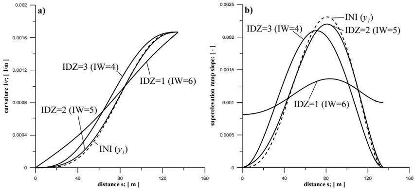
Fig. 5: Route 3 - features of TCs: a) curvatures of the initial and optimised TCs, b) superelevation ramps' slopes
