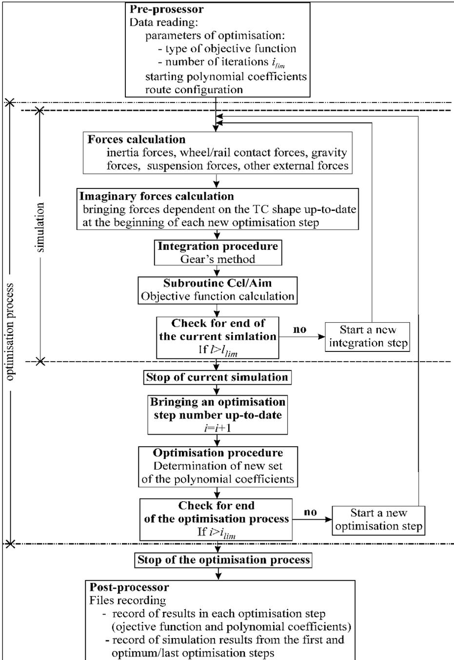
Fig. 2. General scheme of the software to optimise transition curves' shape
