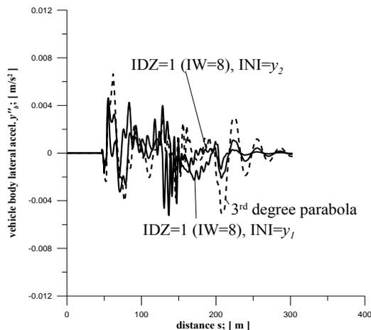
Fig. 14: Results of simulation for vehicle body (lateral acceleration) for the optimised TCs and 3<sup>rd</sup> degree parabola: 10<sup>th</sup> (Routes 5 and 6)
