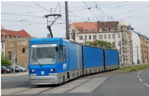
Fig. 2. Example of a three-section tram for urban freight (Hinčica, 2022)
