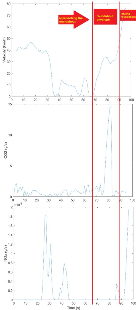
Fig. 8. Example data for PEMS journey at researched roundabout for the parameter of velocity, CO<sub>2</sub> and NO<sub>x</sub> emission
