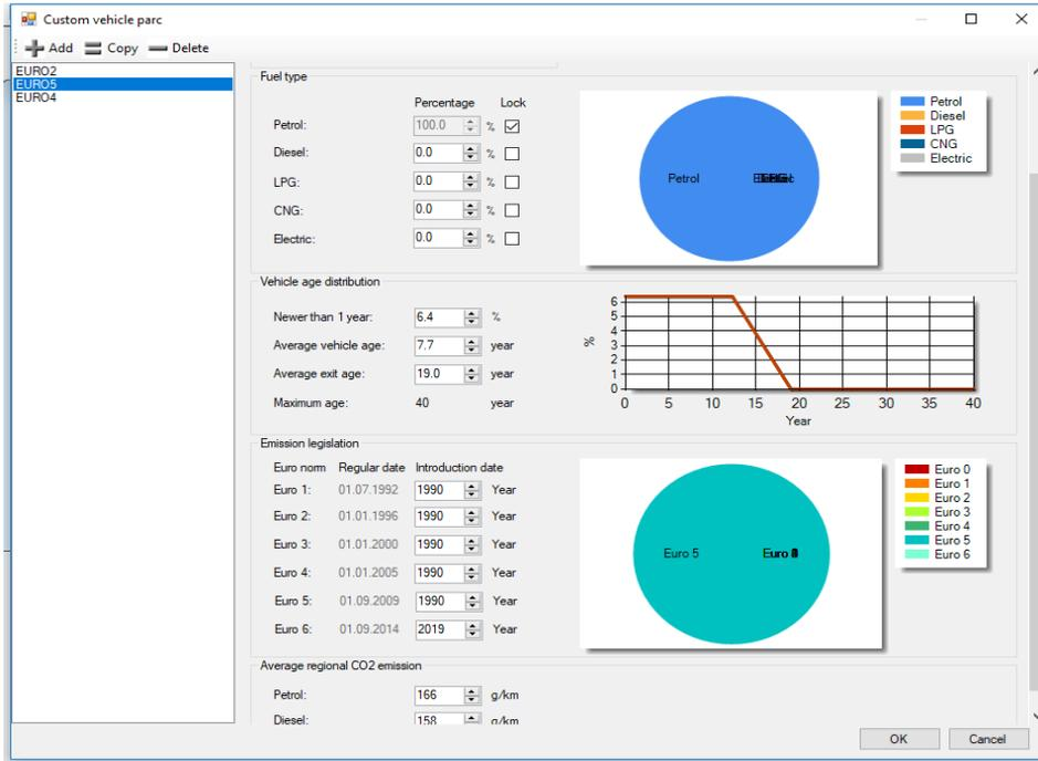
Fig. 7. Example parameter settings for Euro 5 vehicle in the VERSIT+ model
