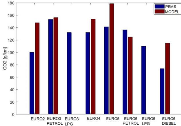
Fig. 12. Comparison of the CO<sub>2</sub> emission from PEMS tests and model data
