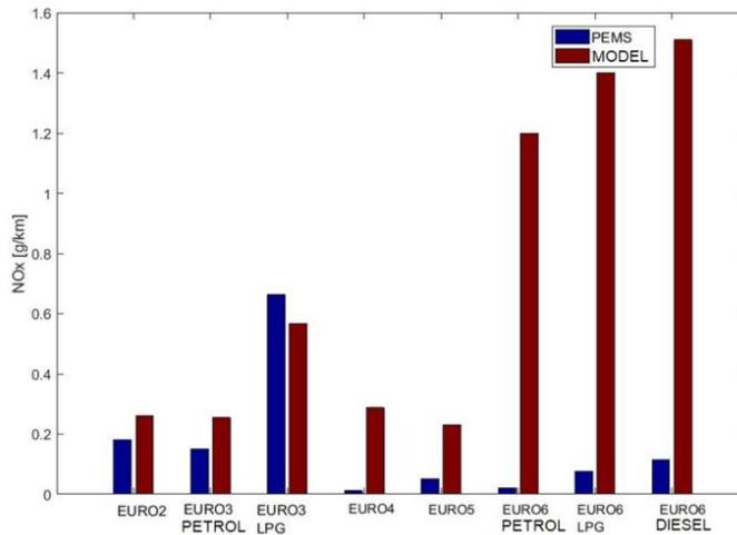
Fig. 13. Comparison of the NO<sub>x</sub> emission from PEMS tests and model data
