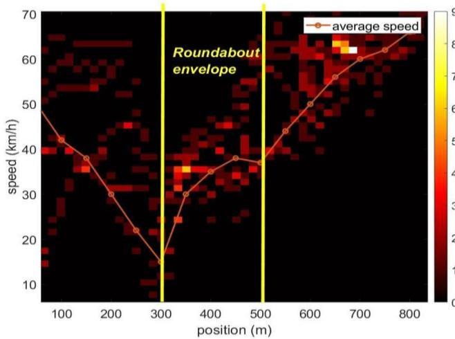
Fig. 9. Average speed profile frequency from road tests for the researched roundabout
