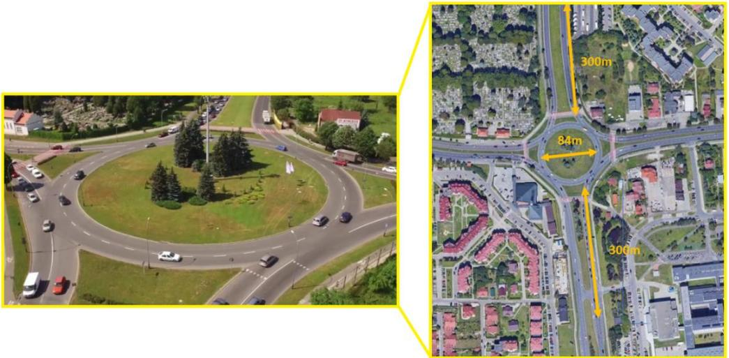
Fig. 5. The researched two-lane roundabout (left) and the map of it (right; with marked outer diameter and researched area)
