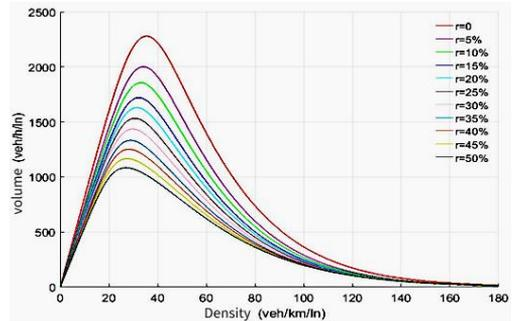
Fig. 2. Volume–density curves derived under different heavy vehicle ratios
