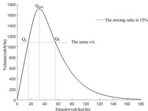
Fig. 4. Volume–density curve when the heavy vehicle mixing ratio is 15%
