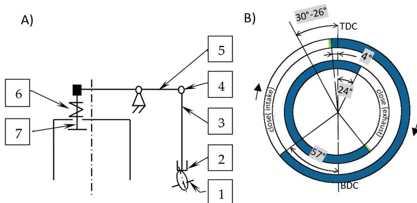
Fig. 2. Schema of classic timing gear engine (A) and schema of timing in engine (B); 1 – timing gear shaft, 2 – cam follower, 3 – cam follower stick, 4 – screw mechanism for regulation of valve clearance, 5 – valve lever, 6 – valve spring, 7 – valve; BDC – bottom dead center, TDC – top dead center
