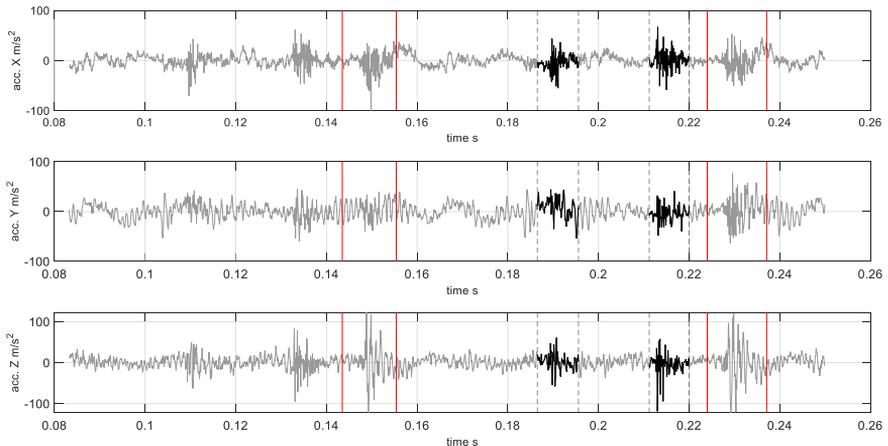
Fig. 5. Example tracings of the vibration accelerations recorded in the X, Y and Z directions – fragment; darker shades and dashed vertical lines denote the closing of the valves, solid vertical lines denote the ignition and combustion
