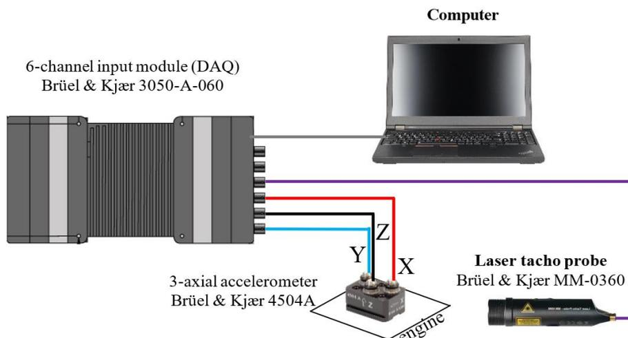
Fig. 3. Diagram of the measurement system used in the measurement of the cylinder head vibration during engine operation
