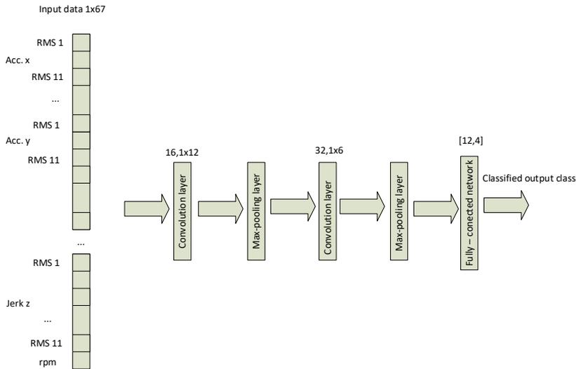
Fig. 8. Structure of the convolutional network used in the recognition of the valve clearance (engine load not included)
