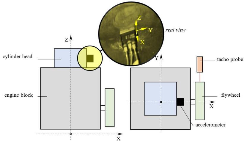
Fig. 4. Measurement directions of the vibration on the cylinder head with the vibration accelerometer fitted on the cylinder head
