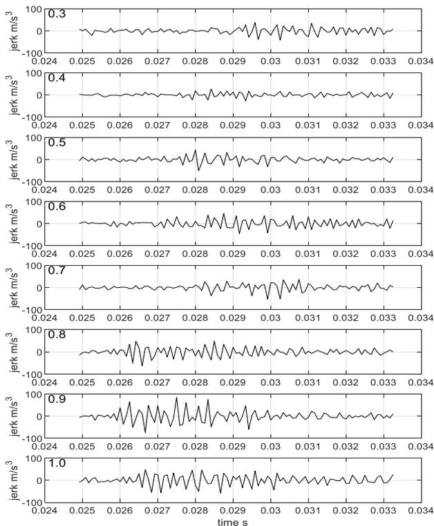
Fig. 6. The response signal to the shock resulting from the impact of the valve on the valve seat for one of the engine valves and different valve clearances
