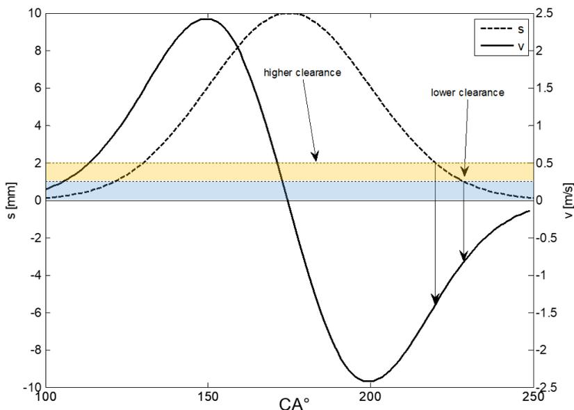
Fig. 1. Changes in the velocity of the impact of the valve on the valve seat in a combustion engine resulting from the change of the valve clearance, CA – crankshaft angle,  $s$  – cam lift,  $v$  – velocity of the point on the cam
