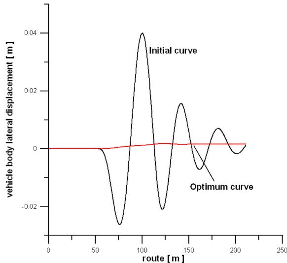
Fig. 9. Dynamical characteristics: (a) vehicle body lateral displacements
