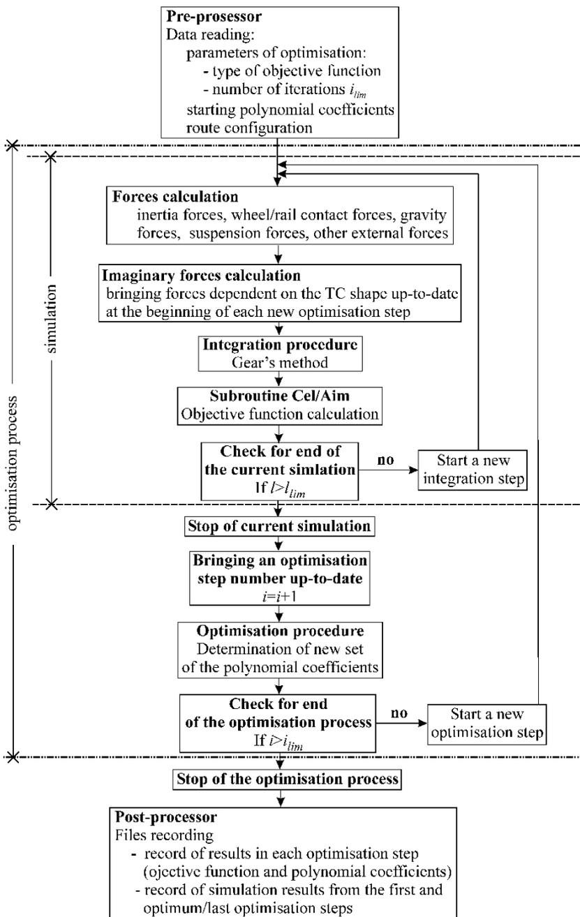
Fig. 2. The scheme of software
