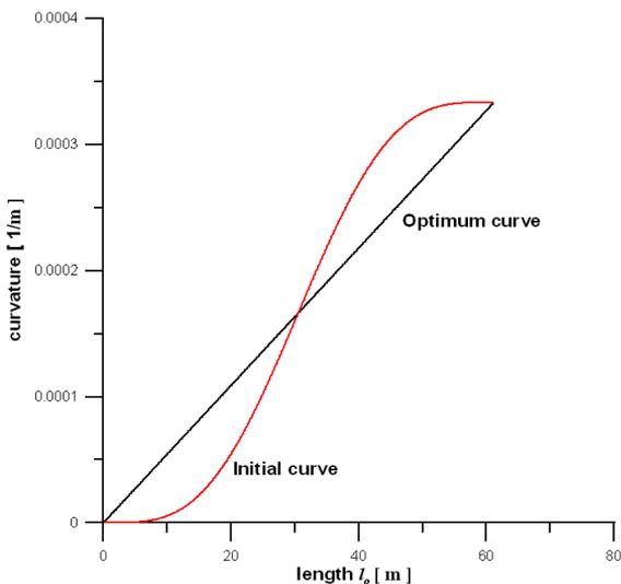
Fig. 8. Transitions curves: (a) curve offsets curvatures
