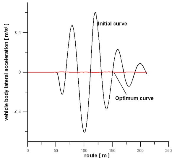
Fig. 10. Dynamical characteristics: vehicle body lateral accelerations
