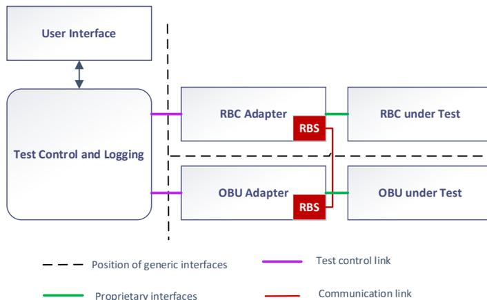
Fig. 5. Architecture of the test environment according to UNISIG (source: own study based on (ERA, 2016d))
