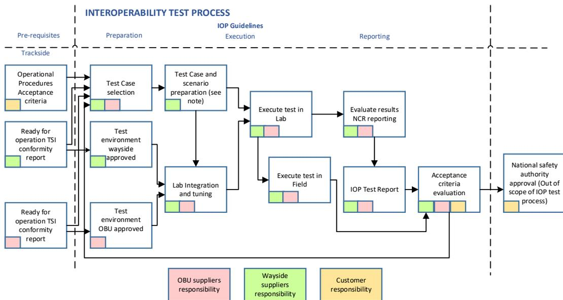
Fig. 4. The IOP testing process according to UNISIG (Subset-110) (source: own study based on (ERA, 2016c))
