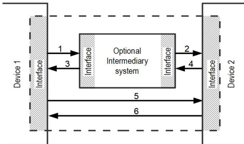
Fig. 1. The idea of cooperation of railway traffic control devices. 1-6 - possible interactions. Source [11].
