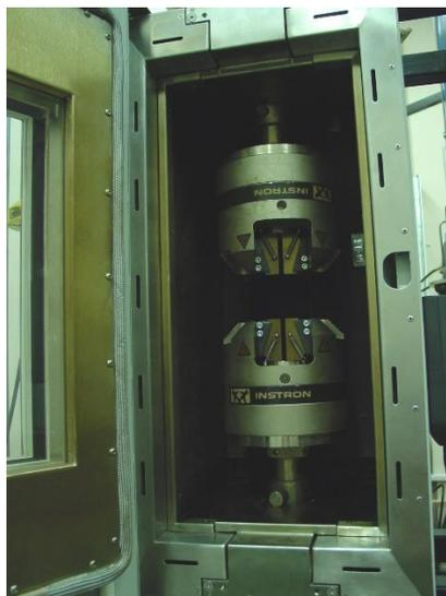
Fig. 2. Instron 8802 strength testing machine with climatic chamber Instron 3119-406-222
