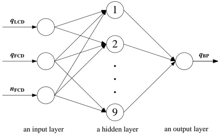
Fig. 1. Structure of weighted traffic flow fusion model of road network
