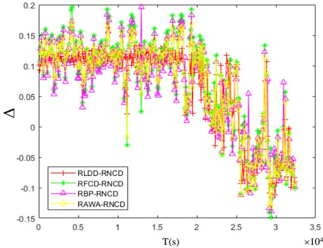
Fig. 8. The difference of the state ratio of road network's MFD obtained by various estimation methods compared with NCD estimation method
