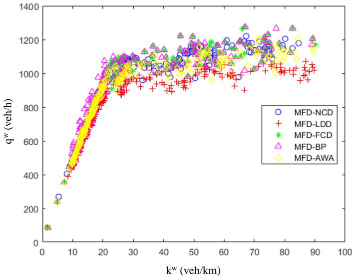
Fig. 6. The two dimensional MFD of road network obtained by various estimation methods
