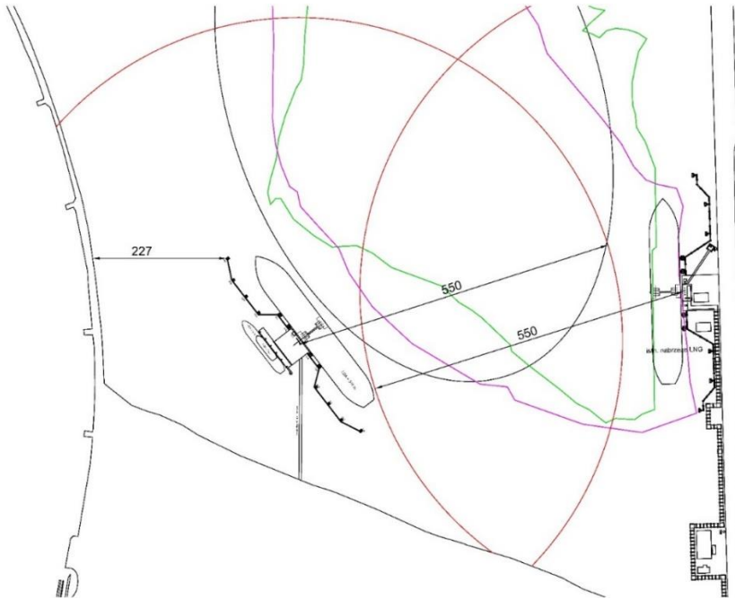
Fig. 2. Preliminary location of the universal LNG transshipment facility and the existing LNG discharge berth
