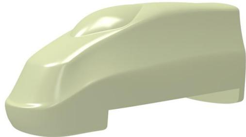
Fig. 5. Surfaces of the crocodile bionic electric locomotive head
