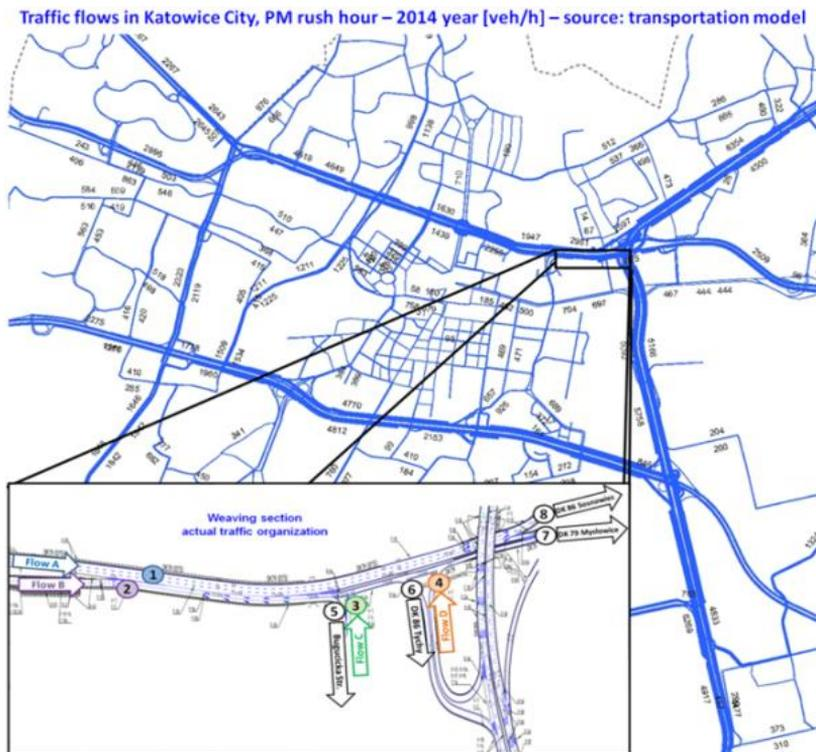
Fig. 4. Location of analyzed weaving section in transportation network – traffic flows estimated from urban transportation model for PM rush hour
