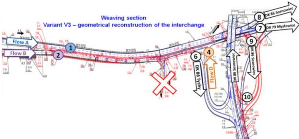
Fig. 5. The most effective solution for example (Wnuk and Karoń, 2014) with geometry changes of interchange
