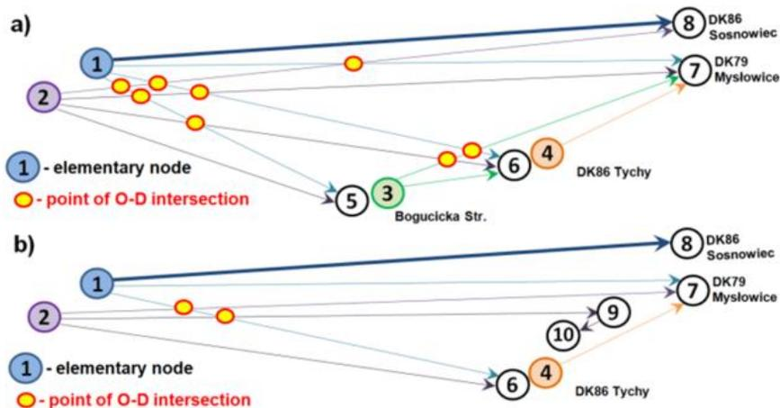
Fig. 6. Weaving diagrams: a) current weaving of traffic flows with eight points of origin-destination (O-D) intersections, b) most effective solution with only two points O-D intersections.
