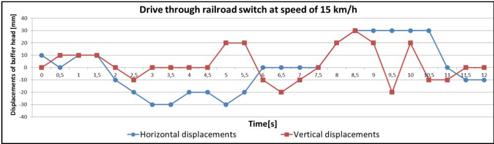
Fig. 8. Displacements of buffer head at speed of 15 km/h
