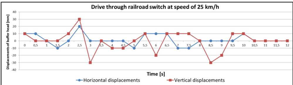
Fig. 11. Displacements of buffer head at speed of 25 km/h (first measurement)
