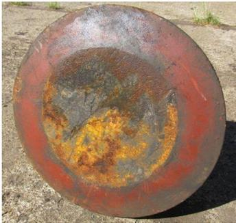
Fig.2. Wear of buffer head
