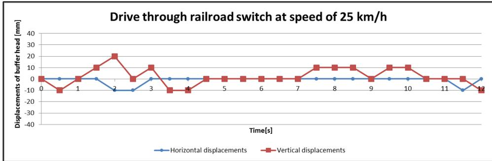
Fig. 12. Displacements of buffer head at speed of 25 km/h (second measurement)
