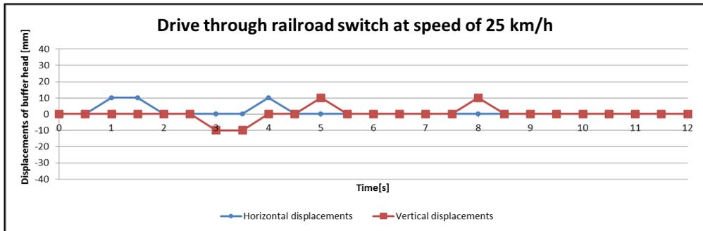
Fig. 13. Displacements of buffer head at speed of 25 km/h (third measurement)
