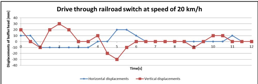
Fig. 10. Displacements of buffer head at speed of 20 km/h (second measurement)
