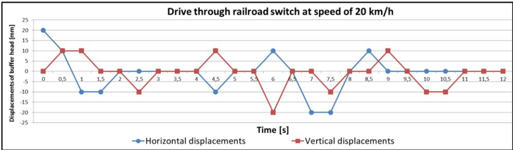
Fig. 9. Displacements of buffer head at speed of 20 km/h (first measurement)
