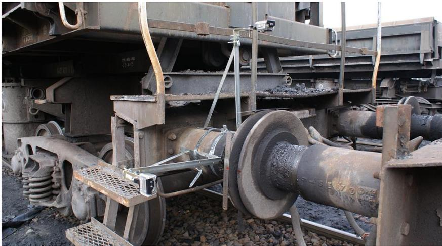
Fig. 3. Mounting location of cameras on buffer
