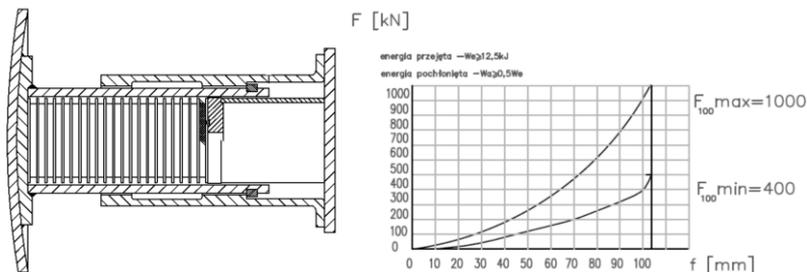
Fig. 4. Cross-section and static characteristic of rubber railway buffer
