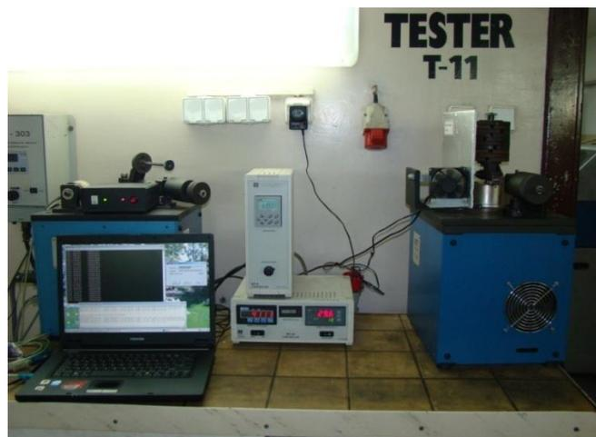
Fig. 1. The T-11 tribological test stand
