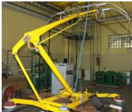
Fig. 4. Test stand for testing of current collectors
