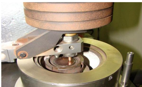
Fig. 3. View on samples during friction testing
