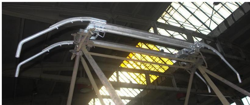
Fig. 11. Testing collector shoe installed on the pantograph
